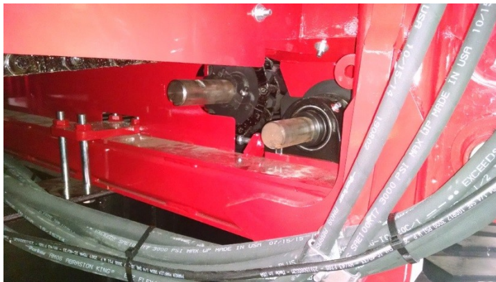
Figure 9-2: Feed Roller and Center Floor Drive Shafts
