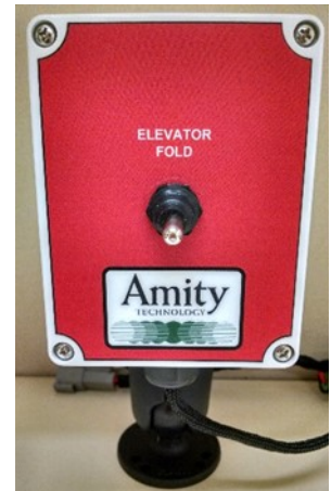
Figure 4-2: Elevator Control Box
