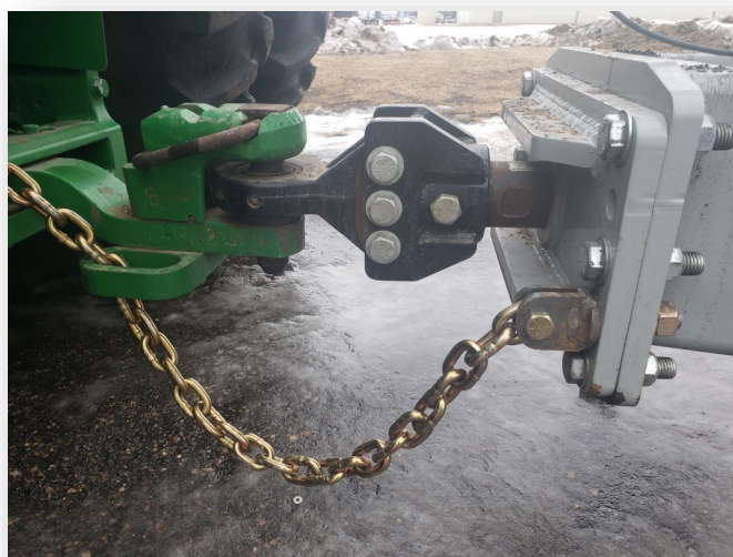
Figure 5-2: Attaching Cart to Tractor Drawbar
